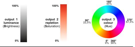
Output 1 = brightness (dimming from dark to a colour) Output 2 = saturation (dimming from white to a colour) Output 3 = colour (0-100% provides all colours) Output 4 = white
