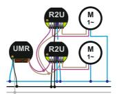
Some types of motors may not be operated parallel, the same goes for operating over the LCN-UMR! You have to seperate the motors, e.g. by using auxiliary relays LCN-R2U!
